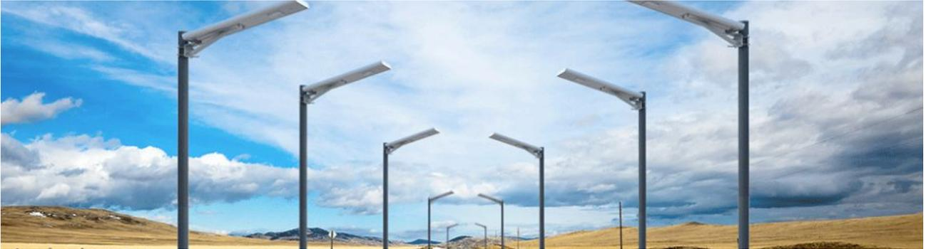
Solar street lights are raised light sources which are powered by photovoltaic panels generally mounted on the lighting structure or integrated in the pole itself. The photovoltaic panels charge a rechargeable battery, which powers a LED lamp during the night.
